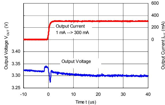
RP508K331x ( $V_{IN} = 5.0$  V,  $V_{OUT} = 3.3$  V)
