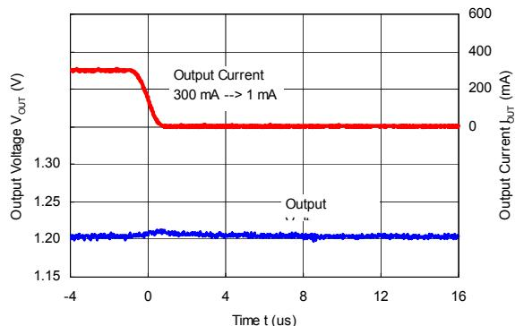
RP508K121x ( $V_{IN} = 3.6 V$ ,  $V_{OUT} = 1.2 V$ )
