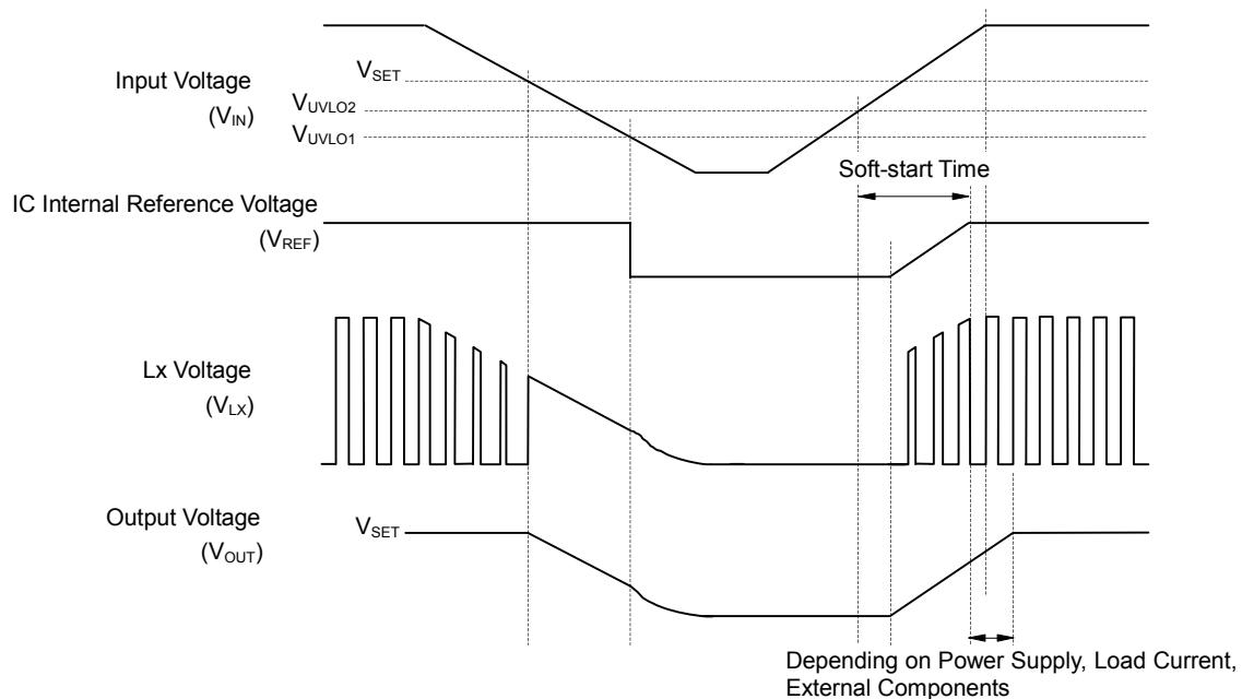
Falling edge (operating) and rising edge (releasing) waveforms of  $V_{OUT}$  could be affected by the initial voltage of  $C_{OUT}$  and the output current of  $V_{OUT}$ .
