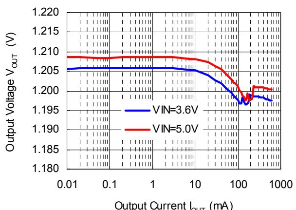
RP508K081x,  $V_{OUT} = 0.8 \text{ V}$
