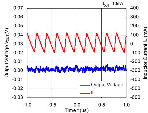
RP508K121x,  $V_{OUT} = 1.2 \text{ V}$  ( $V_{IN} = 3.6 \text{ V}$ )
