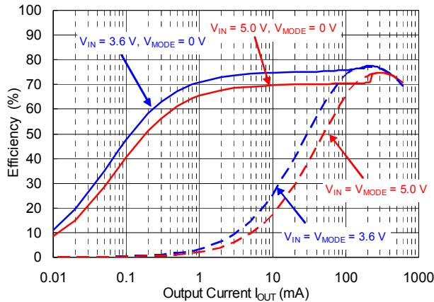
RP508K101x,  $V_{OUT} = 1.0 \text{ V}$
