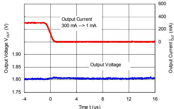
RP508K181x ( $V_{IN} = 3.6\text{ V}$ ,  $V_{OUT} = 1.8\text{ V}$ )
