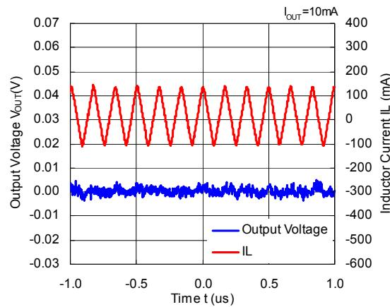
RP508K331x,  $V_{OUT} = 3.3 V$  ( $V_{IN} = 4.3 V$ )
