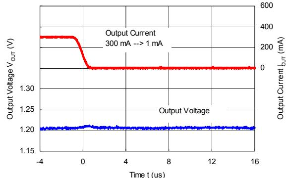
RP508K121x ( $V_{IN} = 3.6 \text{ V}$ ,  $V_{OUT} = 1.2 \text{ V}$ )
