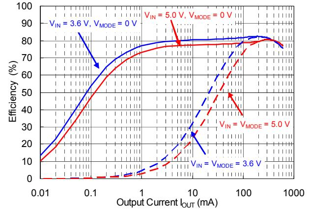
RP508K121x,  $V_{OUT} = 1.2 \text{ V}$
