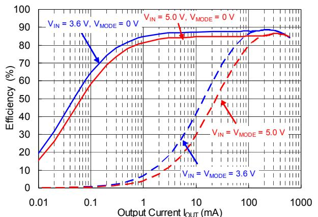
RP508K331x,  $V_{OUT} = 3.3 \text{ V}$
