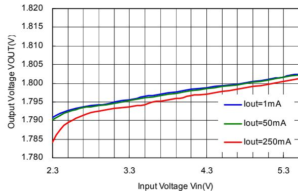
RP508K331x,  $V_{OUT} = 3.3\text{ V}$
