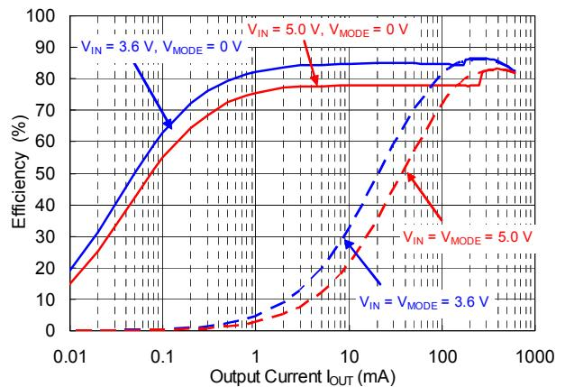
RP508K331x,  $V_{OUT} = 3.3 \text{ V}$
