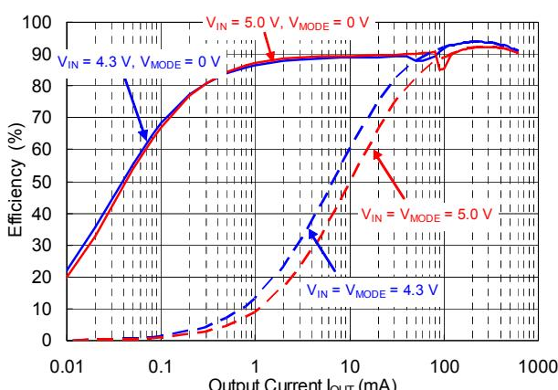
RP508K081x,  $V_{OUT} = 0.8 \text{ V}$
