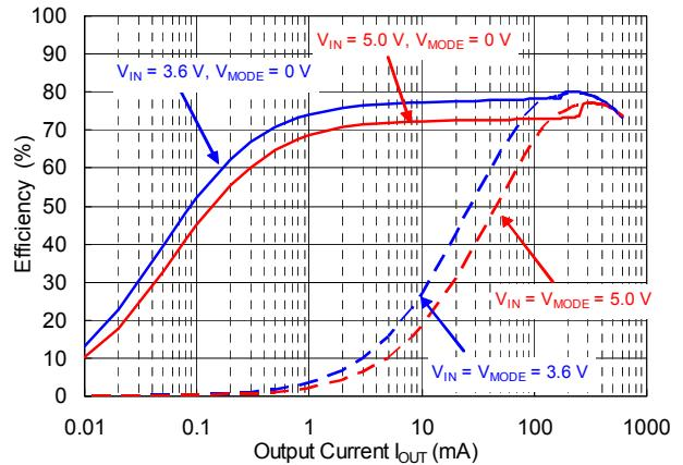
RP508K121x,  $V_{OUT} = 1.2 \text{ V}$
