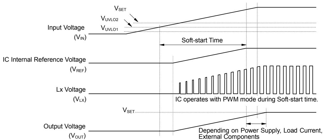
Note that the turn-on speed of  $V_{OUT}$  could be affected by the power supply capacity, the output current, the inductance value, the  $C_{OUT}$  value and the turn-on speed of  $V_{IN}$  determined by  $C_{IN}$ .
