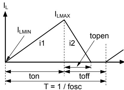
**Figure 2. Inductor Current ( $I_L$ ) flowing through Inductor**
