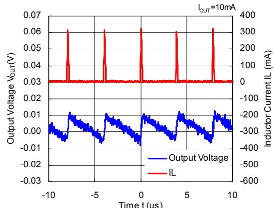
RP508K081x,  $V_{OUT} = 0.8 \text{ V}$  ( $V_{IN} = 3.6 \text{ V}$ )
