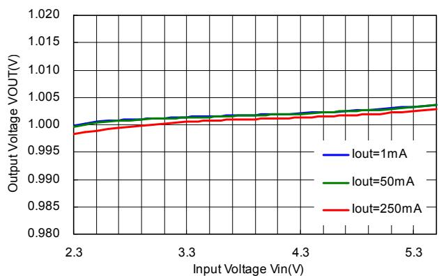
RP508K121x,  $V_{OUT} = 1.2\text{ V}$
