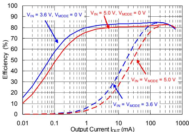
RP508K181x,  $V_{OUT} = 1.8 \text{ V}$
