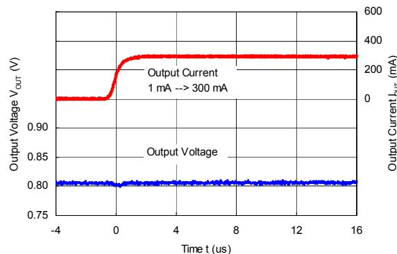
RP508K081x ( $V_{IN} = 3.6$  V,  $V_{OUT} = 0.8$  V)
