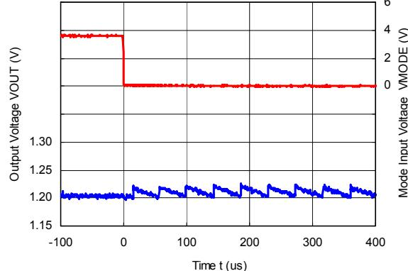
RP508K181x ( $V_{IN} = 3.6 \text{ V}$ ,  $V_{OUT} = 1.8 \text{ V}$ ,  $I_{OUT} = 1 \text{ mA}$ )
