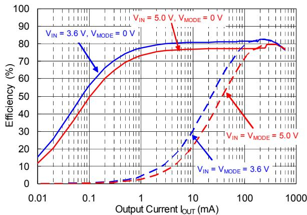
RP508K181x,  $V_{OUT} = 1.8 \text{ V}$
