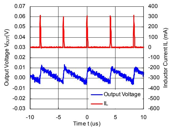
RP508K121x,  $V_{OUT} = 1.2 \text{ V}$  ( $V_{IN} = 3.6 \text{ V}$ )
