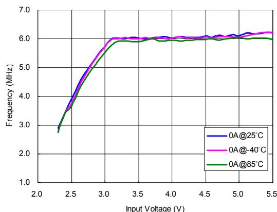
RP508K181x,  $V_{OUT} = 1.8 V$  ( $V_{IN} = 3.6 V$ )
