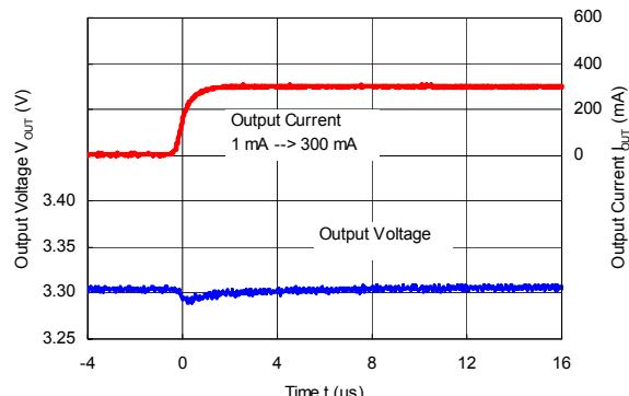
RP508K331x ( $V_{IN} = 5.0\text{ V}$ ,  $V_{OUT} = 3.3\text{ V}$ )
