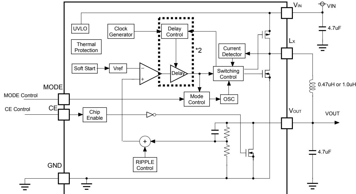
Switching frequency in order to become reference frequency (6 MHz), delay time is included the output voltage feedback loop and locked the frequency (6 MHz).
