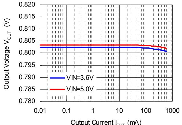
RP508K101x,  $V_{OUT} = 1.0 \text{ V}$
