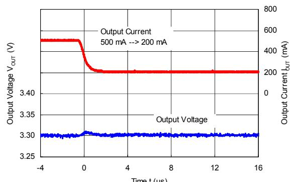
**Load Transient Response ( $C_{OUT} = 4.7\mu F$ , C1005X5R0J475M)**
