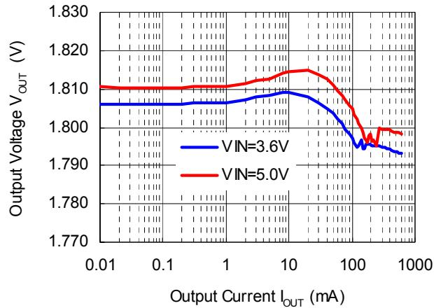
RP508K181x,  $V_{OUT} = 1.8$  V
