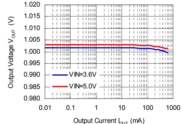
RP508K121x,  $V_{OUT} = 1.2 \text{ V}$
