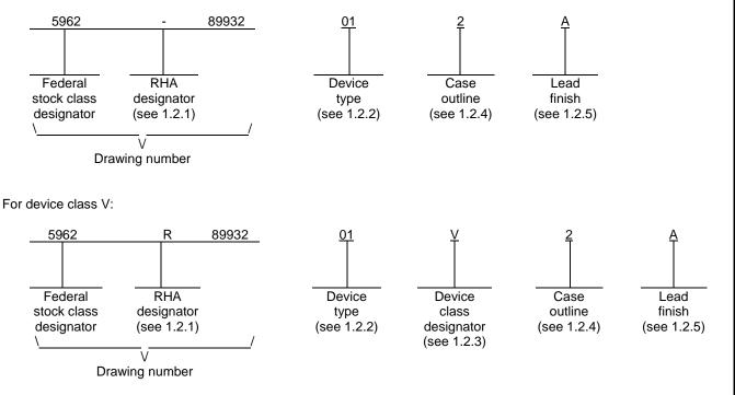
1.2.1 <u>RHA designator</u>. Device classes Q and V RHA marked devices meet the MIL-PRF-38535 specified RHA levels and are marked with the appropriate RHA designator. Device class M RHA marked devices meet the MIL-PRF-38535, appendix A specified RHA levels and are marked with the appropriate RHA designator. A dash (-) indicates a non-RHA device.
