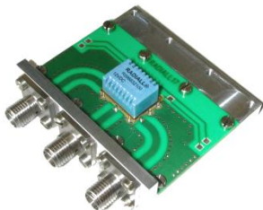
Relay soldered on Test Fixture (2)
