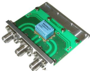
Relay soldered on Test Fixture (2)
