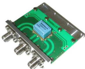
Relay soldered on Test Fixture (2)
