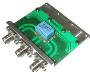
Relay soldered on Test Fixture (2)
