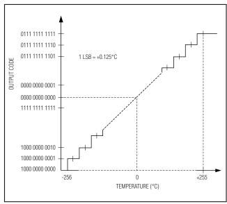
Figure 14. Temperature Transfer Function
