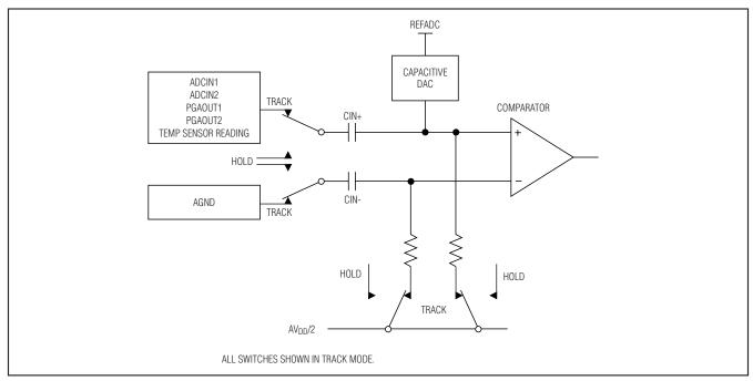
Figure 12. Analog Input Track and Hold
