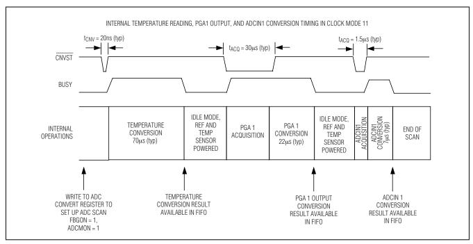
Figure 15. ADC Clock Mode 11 Example
