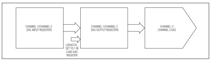
Figure 16. DAC Functional Diagram
