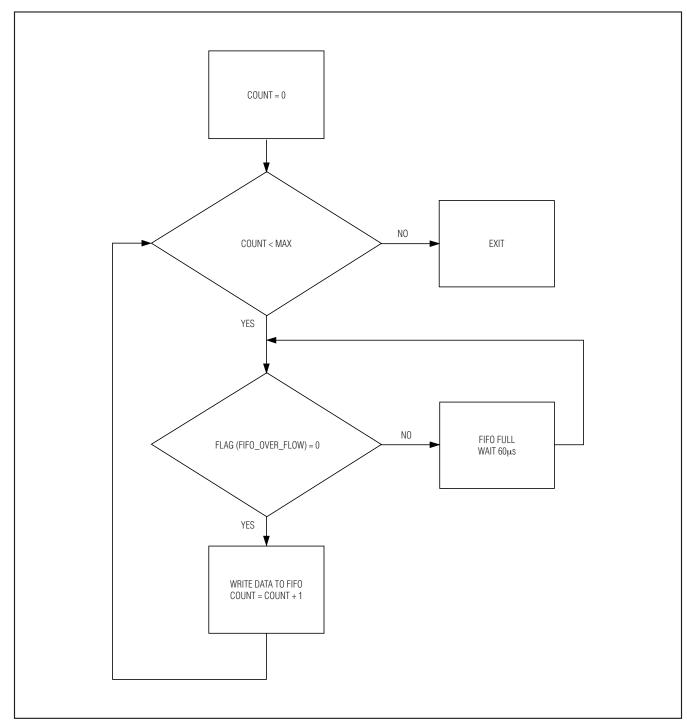
Figure 17. Software Flow Control Example (Pseudo Code)
