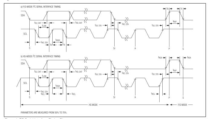
Figure 4. I<sup>2</sup>C Serial-Interface Timing Diagram
