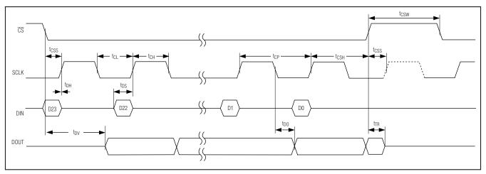
Figure 1. SPI Serial-Interface Timing
