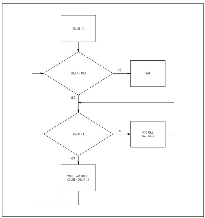
Figure 18. Hardware Flow Control Example (Pseudo Code)
