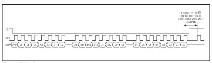
Figure 2. SPI Write Sequence
