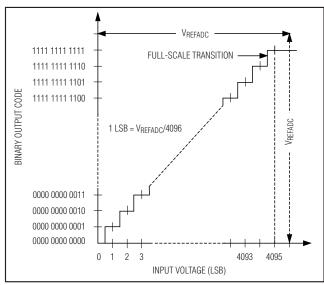
Figure 13. ADC Transfer Function
