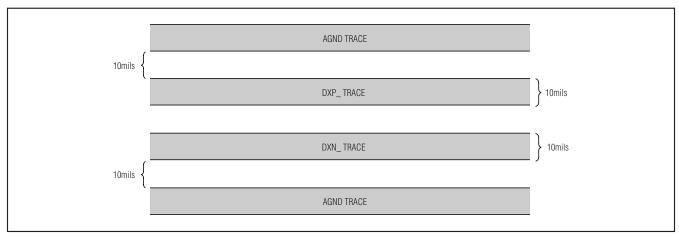
Figure 23. Recommended DXP\_ and DXN\_ PCB Trace Layout
