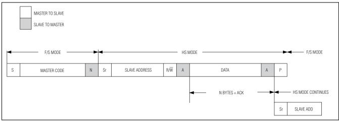
Figure 9. Data-Transfer Format in HS Mode
