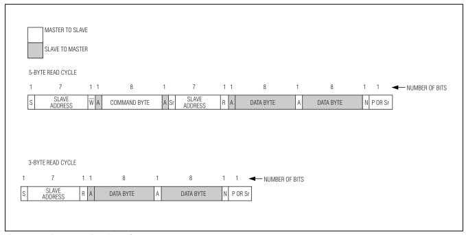
Figure 11. 5-Byte and 3-Byte Read Cycle
