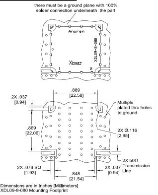
In order for Xinger surface mount delay lines to work optimally, there must be  $50\Omega$  transmission lines leading to and from all of the RF ports. Also, there must be a very good ground plane under the part with a number of plated thru holes to ensure proper electrical performance. If any of these conditions are not satisfied, insertion loss, average delay and VSWR may not meet published specifications.
