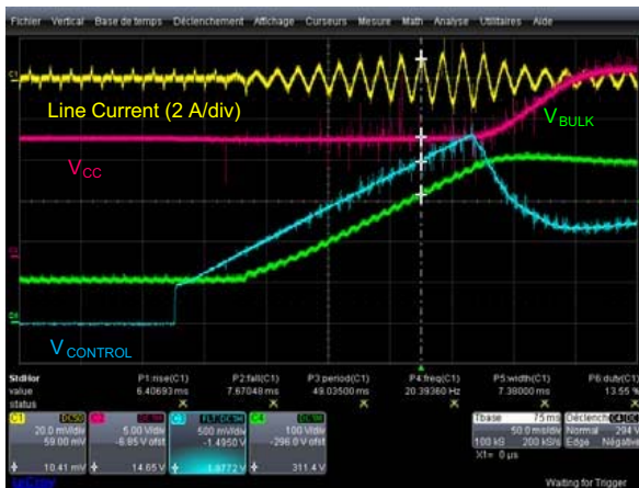
b) Start of operation when V_{in,rms} exceeds (V_{in,rms})_{BOH} (NCP1612A)
