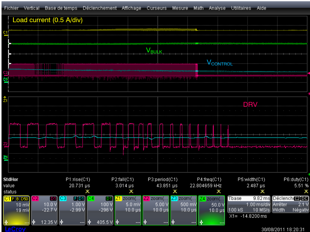
Figure 16. Soft Over-Voltage Protection
