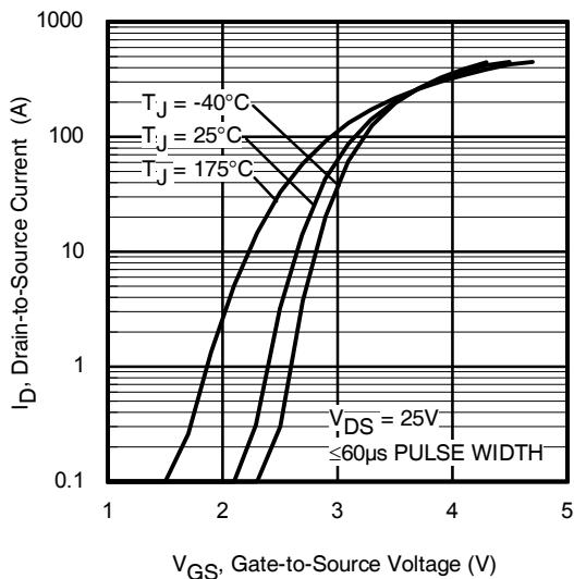
**Fig. 5.** Transfer Characteristics
