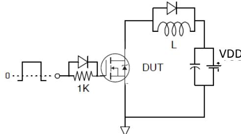
Fig 19a. Gate Charge Test Circuit
