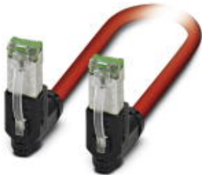
SERCOS III patch cable, shielded, star quad, AWG 22 stranded (7-wire), RAL 3020 (traffic red), RJ45 connector/IP 20, angled, to RJ45 connector/IP20, angled, length: 2.0 m
