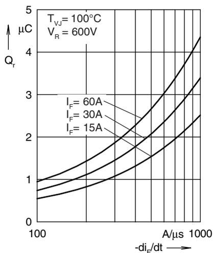
Fig. 2 Reverse recovery charge  $Q_r$  versus  $-di_F/dt$
