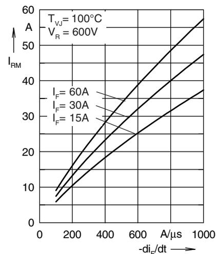
Fig. 3 Peak reverse current  $I_{RM}$  versus  $-di_F/dt$
