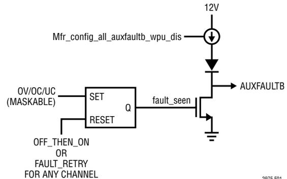
Figure 1. AUXFAULTB MUX
