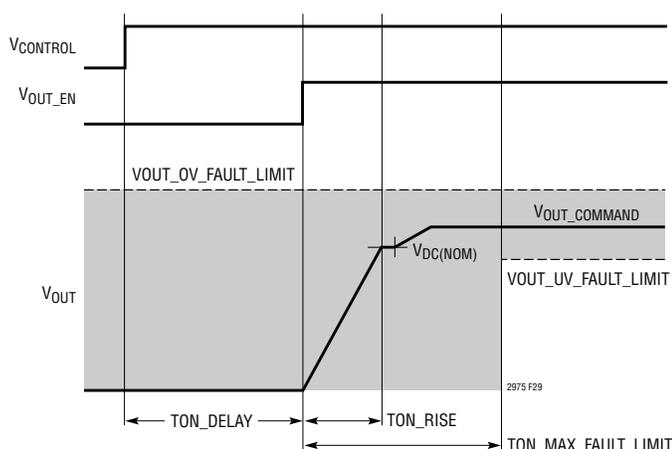
Figure 29. Typical ON Sequence Using Control Pin
