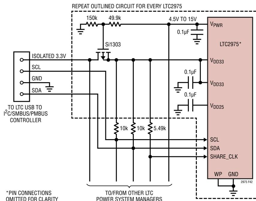
Figure 42. LTC Controller Connections When V<sub>PWR</sub> Is Used
