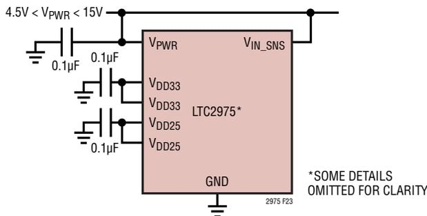
Figure 23. Powering LTC2975 Directly from an Intermediate Bus
