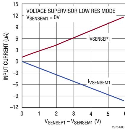
Voltage Sense Differential Input Current vs Differential Input Voltage
