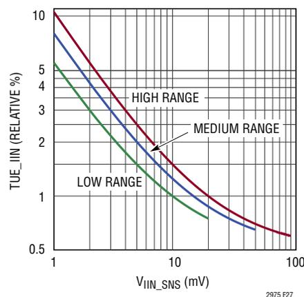
Figure 27.  $TUE\_IIN$  vs  $READ\_IIN$  Input Voltage in Percentage
