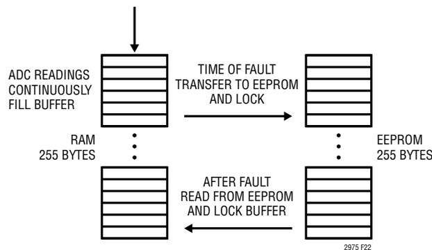
Figure 22. Fault Logging
