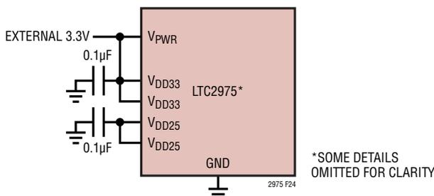
Figure 24. Powering LTC2975 from External 3.3V Supply
