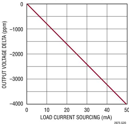
**V<sub>OUT\_EN[0:3]</sub> and AUXFAULTB Output High Voltage vs Load Current**
