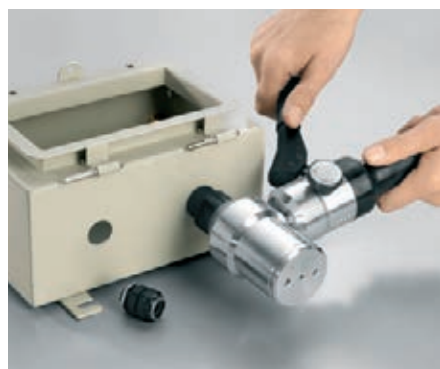
The hydraulic hole puncher punches out precise holes for accommodating metric and PG cable glands.
