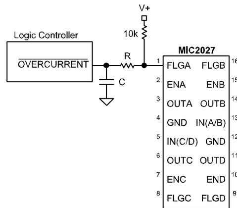
Figure 3. Transient Filter
