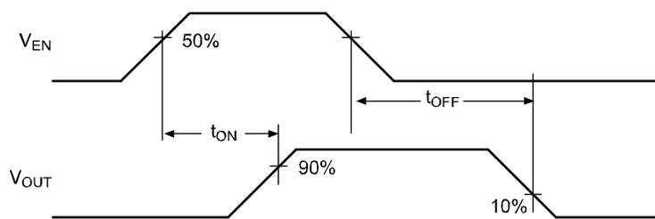
**Active-High Switch Delay Times (MIC20x7-1)**
