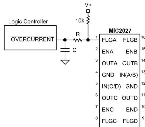
Figure 3. Transient Filter
