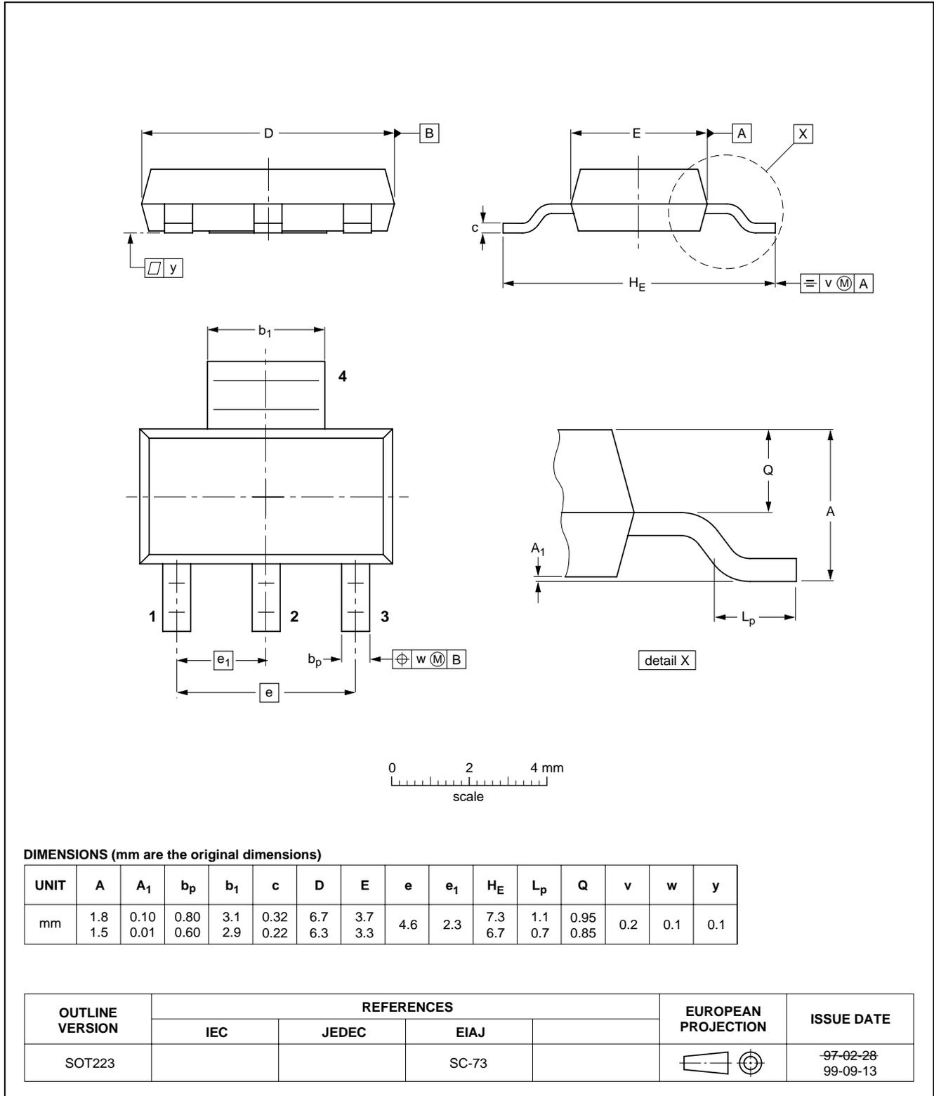
40 V low  $V_{CEsat}$  PNP transistor
