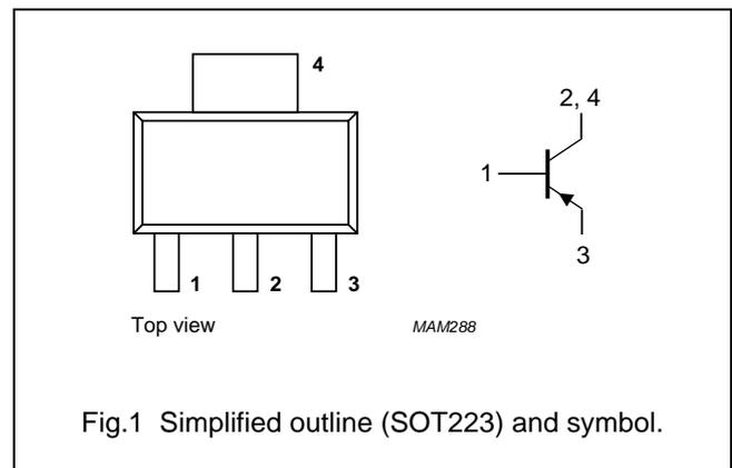
40 V low  $V_{CEsat}$  PNP transistor
