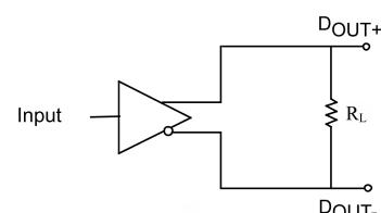
FIGURE 6.  $f_{MAX}$  Test Circuit
