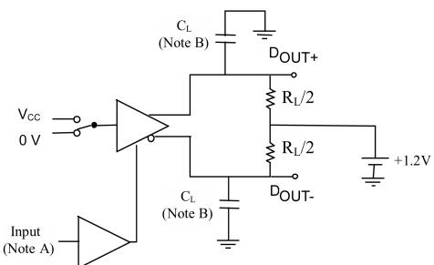
Note B: All input pulses have the frequency = 10 MHz,  $t_R$  or  $t_F$  = 1 ns
