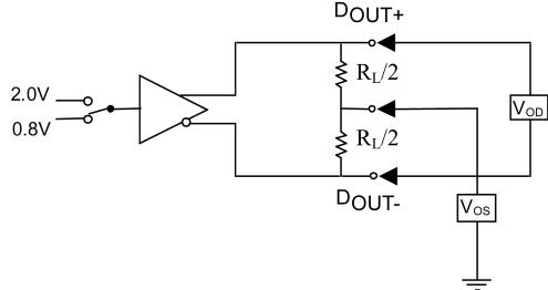
FIGURE 1. Differential Driver DC Test Circuit
