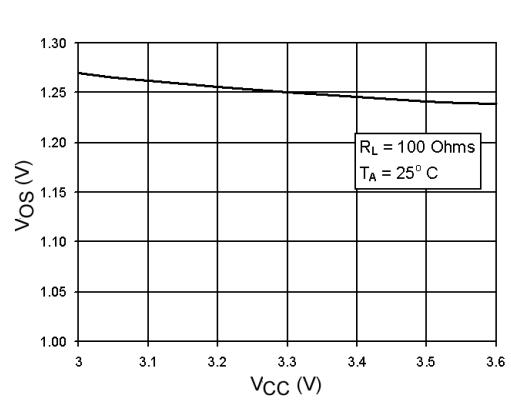
FIGURE 12. Offset Voltage vs.
