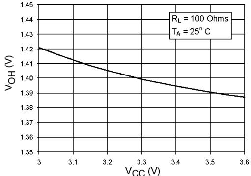
FIGURE 7. Output High Voltage vs.
