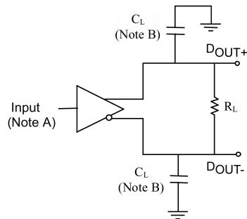
Note A: All input pulses have frequency = 10 MHz,  $t_R$  or  $t_F$  = 1 ns
