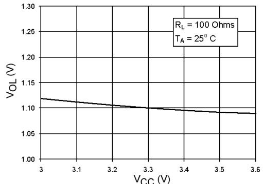
FIGURE 8. Output Low Voltage vs.
