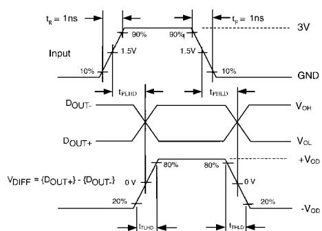
FIGURE 3. AC Waveforms
