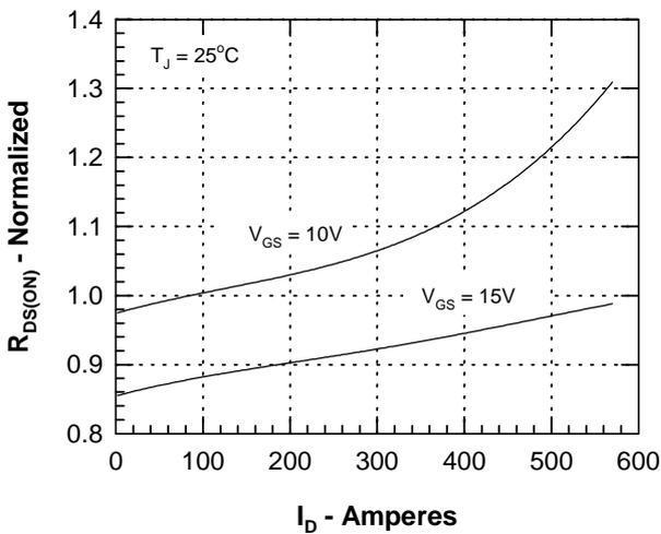
Figure 5.  $R_{DS(on)}$  normalized to  $0.5 I_{D25}$  value
