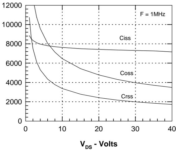
Figure 9. Capacitance Curves
