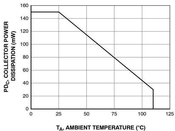
**Figure 1. Collector Power Dissipation vs. Ambient Temperature**
