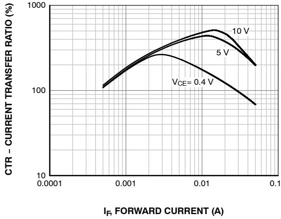
**Figure 10. Current Transfer Ratio vs. Forward Current**
