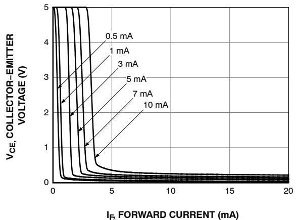
**Figure 5. Collector Emitter Voltage vs. Forward Current**
