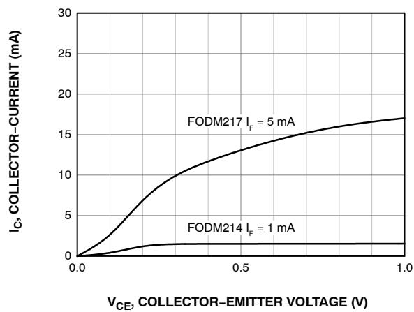
**Figure 7. Collector Current vs. Small Collector-Emitter Voltage**
