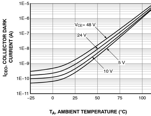
**Figure 9. Collector Dark Current vs. Ambient Temperature**
