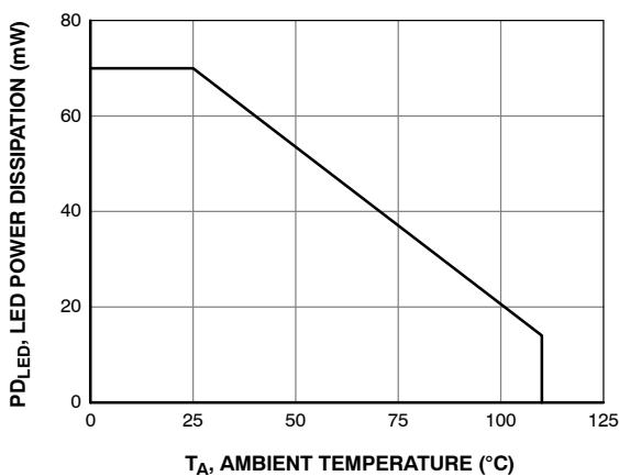
**Figure 2. LED Power Dissipation vs. Ambient Temperature**
