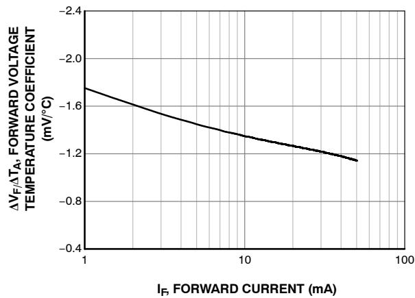
**Figure 4. Forward Voltage Temperature Coefficient vs. Forward Current**
