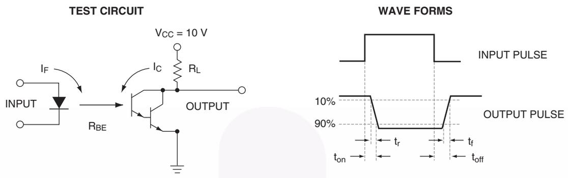
Figure 8. Switching Time Test Circuit and Waveform
