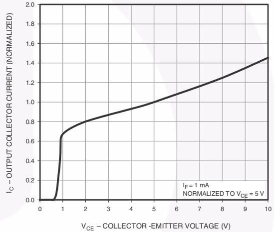
**Figure 6. Output Current vs. Collector - Emitter Voltage**
