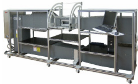
FDK Original Wind Tunnel
