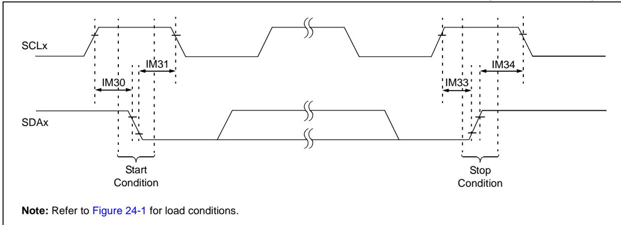
**FIGURE 24-20: I2Cx BUS DATA TIMING CHARACTERISTICS (MASTER MODE)**
