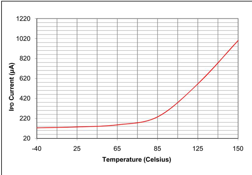
**FIGURE 27-9: TYPICAL I<sub>DOZE</sub> CURRENT @ V<sub>DD</sub> = 3.3V**
