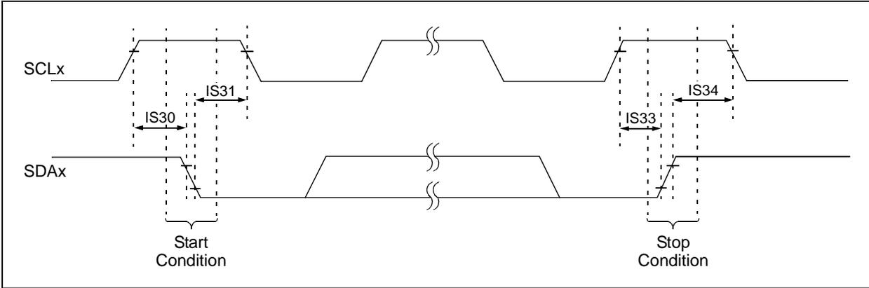
**FIGURE 24-22: I2Cx BUS DATA TIMING CHARACTERISTICS (SLAVE MODE)**
