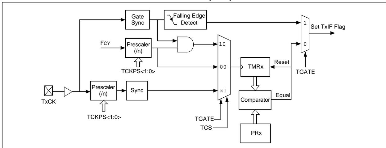
**FIGURE 12-2: TYPE C TIMER BLOCK DIAGRAM (x = 3)**
