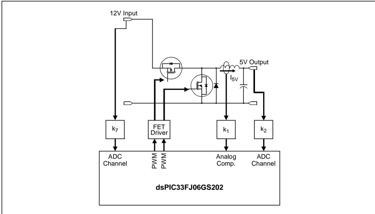
**FIGURE 2-7: MULTI-PHASE SYNCHRONOUS BUCK CONVERTER**
