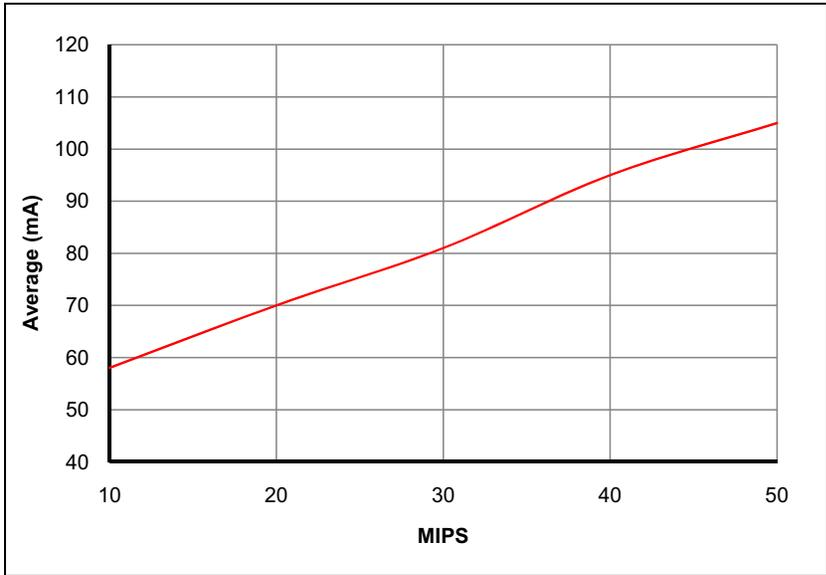
**FIGURE 27-10: TYPICAL I<sub>IDLE</sub> CURRENT @ V<sub>DD</sub> = 3.3V**
