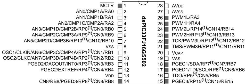
**Note 1:** The RPN pins can be used by any remappable peripheral. See [Table 1](#) for the list of available peripherals.
