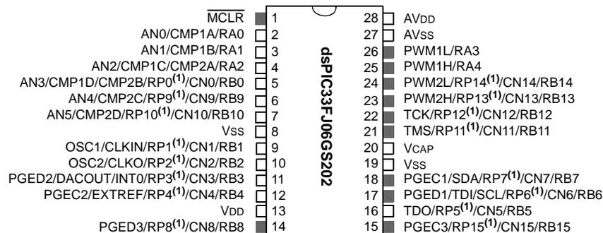
**Note 1:** The RPN pins can be used by any remappable peripheral. See [Table 1](#) for the list of available peripherals.
