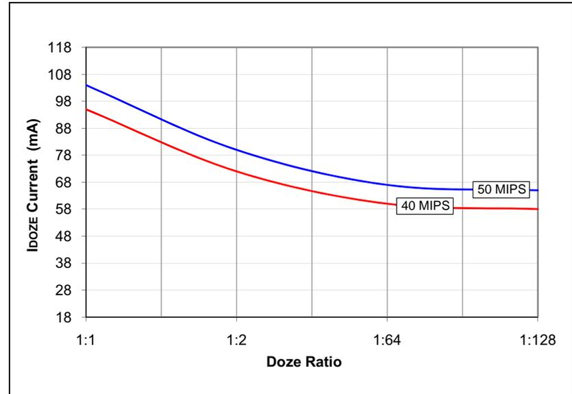
**FIGURE 27-8: TYPICAL I<sub>DD</sub> CURRENT @ V<sub>DD</sub> = 3.3V**
