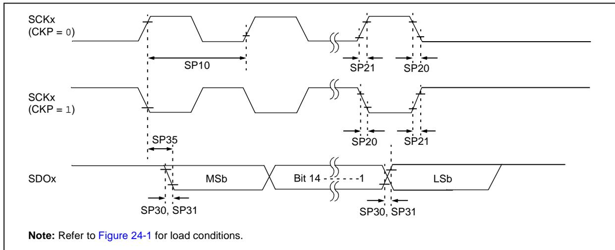
FIGURE 24-12: SPIx MASTER MODE (HALF-DUPLEX, TRANSMIT ONLY, CKE = 1) TIMING CHARACTERISTICS
