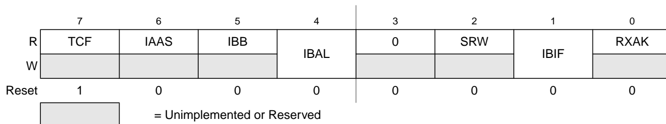
Figure 11-6. IIC Bus Status Register (IBSR)
