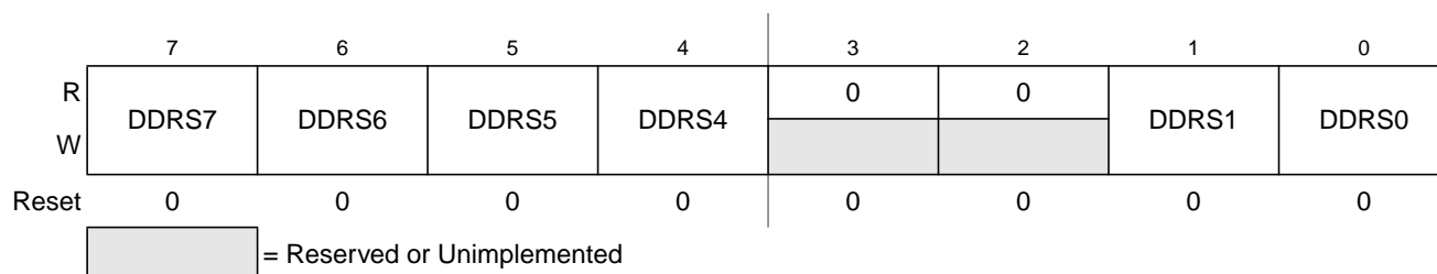
Figure 4-32. Port S Data Direction Register (DDRS)
