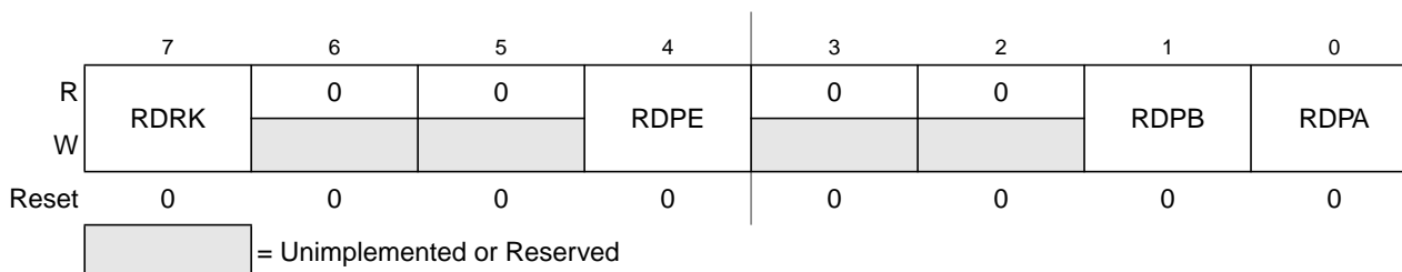
Figure 21-15. Reduced Drive Register (RDRIV)
