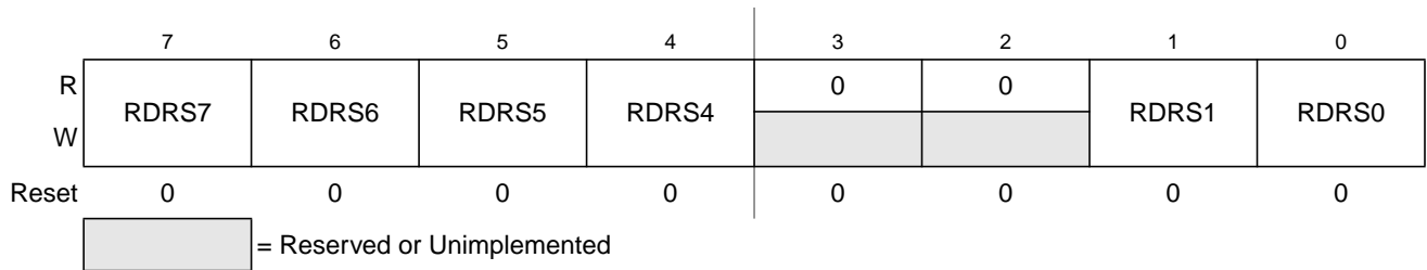
Figure 4-33. Port S Reduced Drive Register (RDRS)
