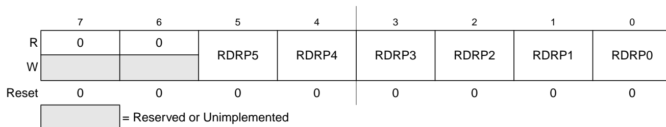
Figure 4-26. Port P Reduced Drive Register (RDRP)
