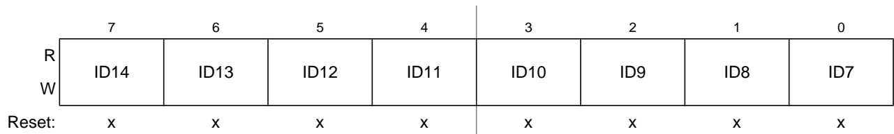
Figure 12-25. Identifier Register 2 (IDR2) — Extended Identifier Mapping
