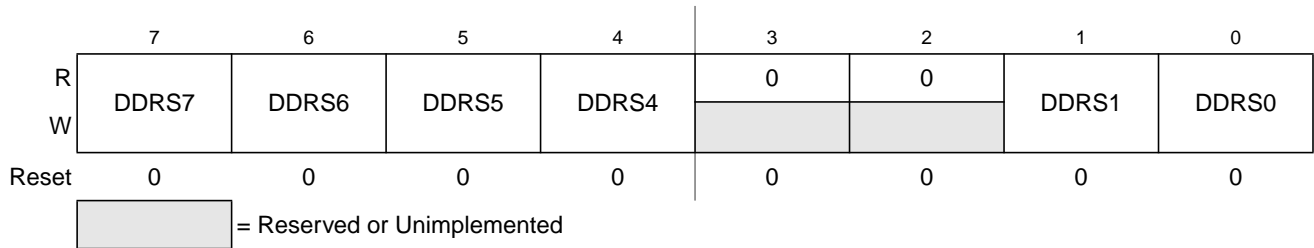
Figure 4-32. Port S Data Direction Register (DDRS)
