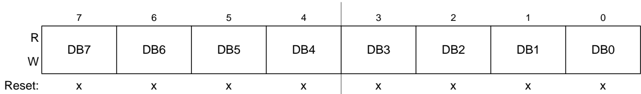
Figure 12-31. Data Segment Registers (DSR0–DSR7) — Extended Identifier Mapping
