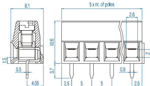
**5.00mm Pin Spacing** – Fixed PCB Blocks
