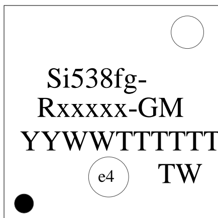
Figure 12.1. Si5381/82 Top Marking
