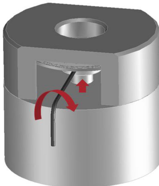
Figure 1d. Tighten the set screws
