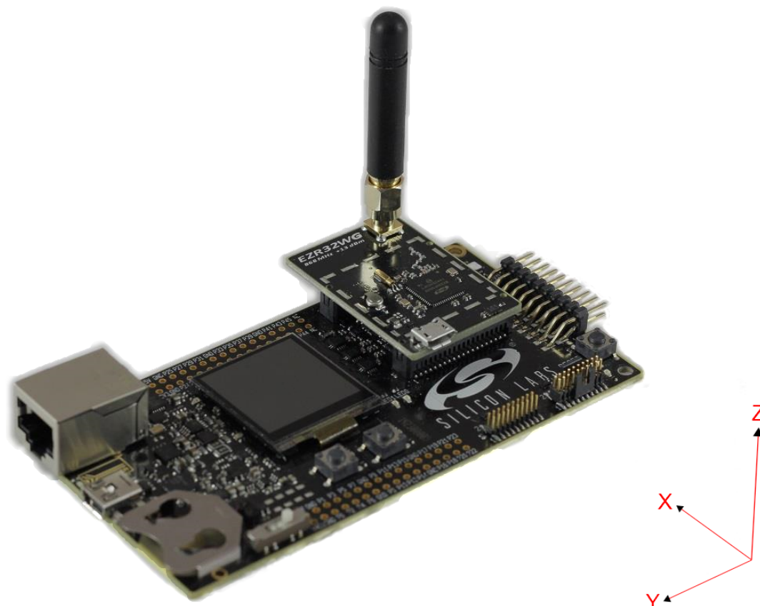
Figure 6.2. DUT: BRD4502C (Rev. A00) Radio Board with Wireless Starter Kit Mainboard
