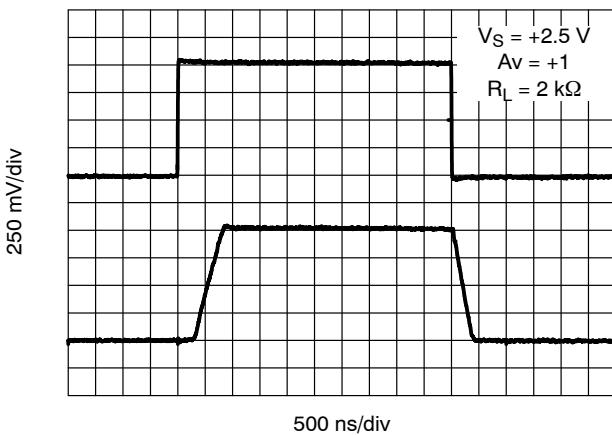
Figure 20. 2.5 V Non-Inverting Large Signal Pulse Response
