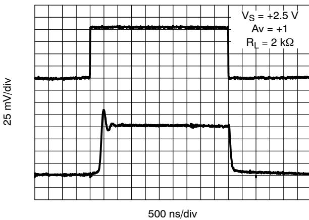
Figure 22. 2.5 V Non-Inverting Small Signal Pulse Response
