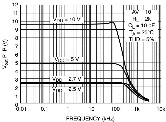
Figure 11. Peak-to-Peak Output vs. Supply vs. Frequency
