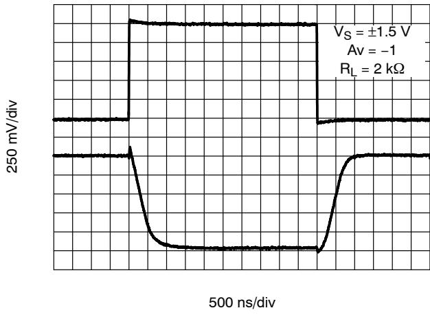
**Figure 23. 3 V Inverting Large Signal Pulse Response**
