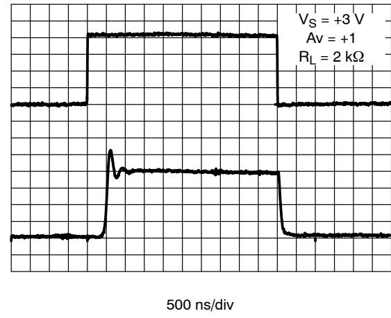
**Figure 26. 3 V Non-Inverting Small Signal Pulse Response**
