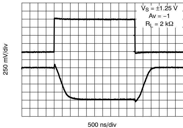
Figure 19. 2.5 V Inverting Large Signal Pulse Response
