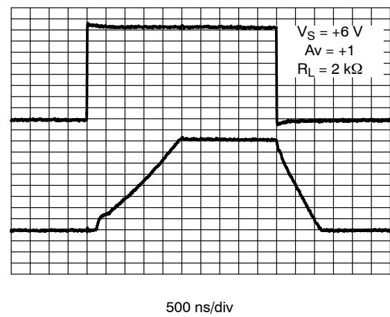
**Figure 28. 6 V Non-Inverting Large Signal Pulse Response**
