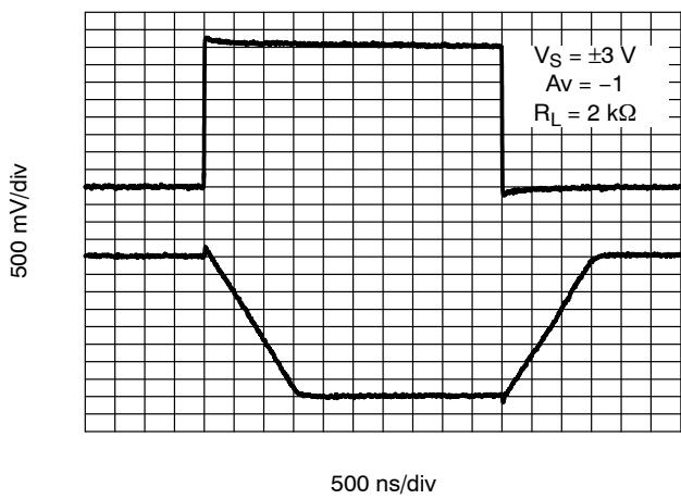
**Figure 27. 6 V Inverting Large Signal Pulse Response**
