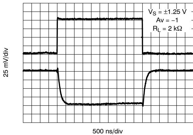
Figure 21. 2.5 V Inverting Small Signal Pulse Response
