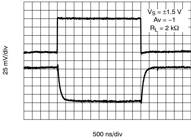
**Figure 25. 3 V Inverting Small Signal Pulse Response**
