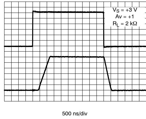
**Figure 24. 3 V Non-Inverting Large Signal Pulse Response**
