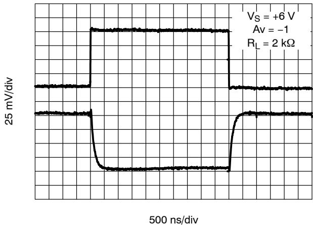
**Figure 29. 6 V Inverting Small Signal Pulse Response**
