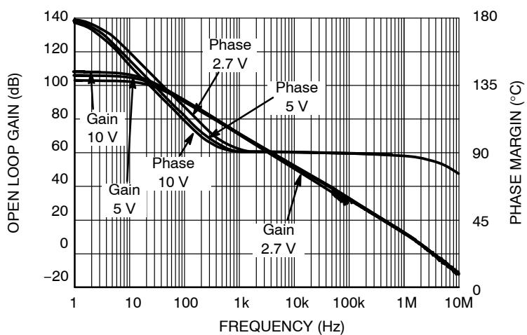
**Figure 14. Open Loop Gain and Phase vs. Frequency**
