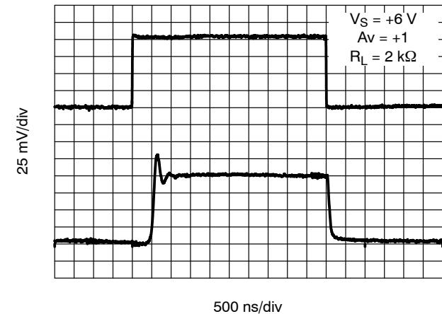
**Figure 30. 6 V Non-Inverting Small Signal Pulse Response**
