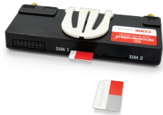
DUAL-SIM SUPPORT WITH UPGRADABLE LTE CELLULAR MODEM
