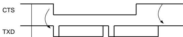
Figure 33-29. Transmitter Behavior when Operating with Hardware Handshaking
