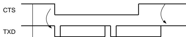
Figure 33-29. Transmitter Behavior when Operating with Hardware Handshaking
