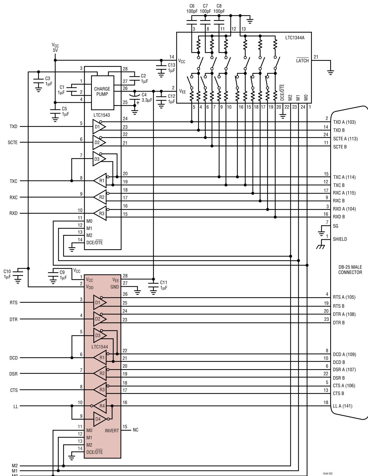
Figure 22. Controller-Selectable Multiprotocol DTE Port with DB-25 Connector
