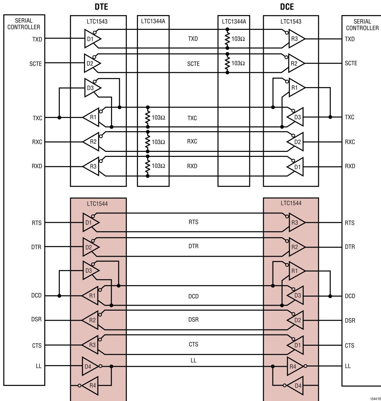
Figure 9. Complete Multiprotocol Interface in EIA530 Mode
