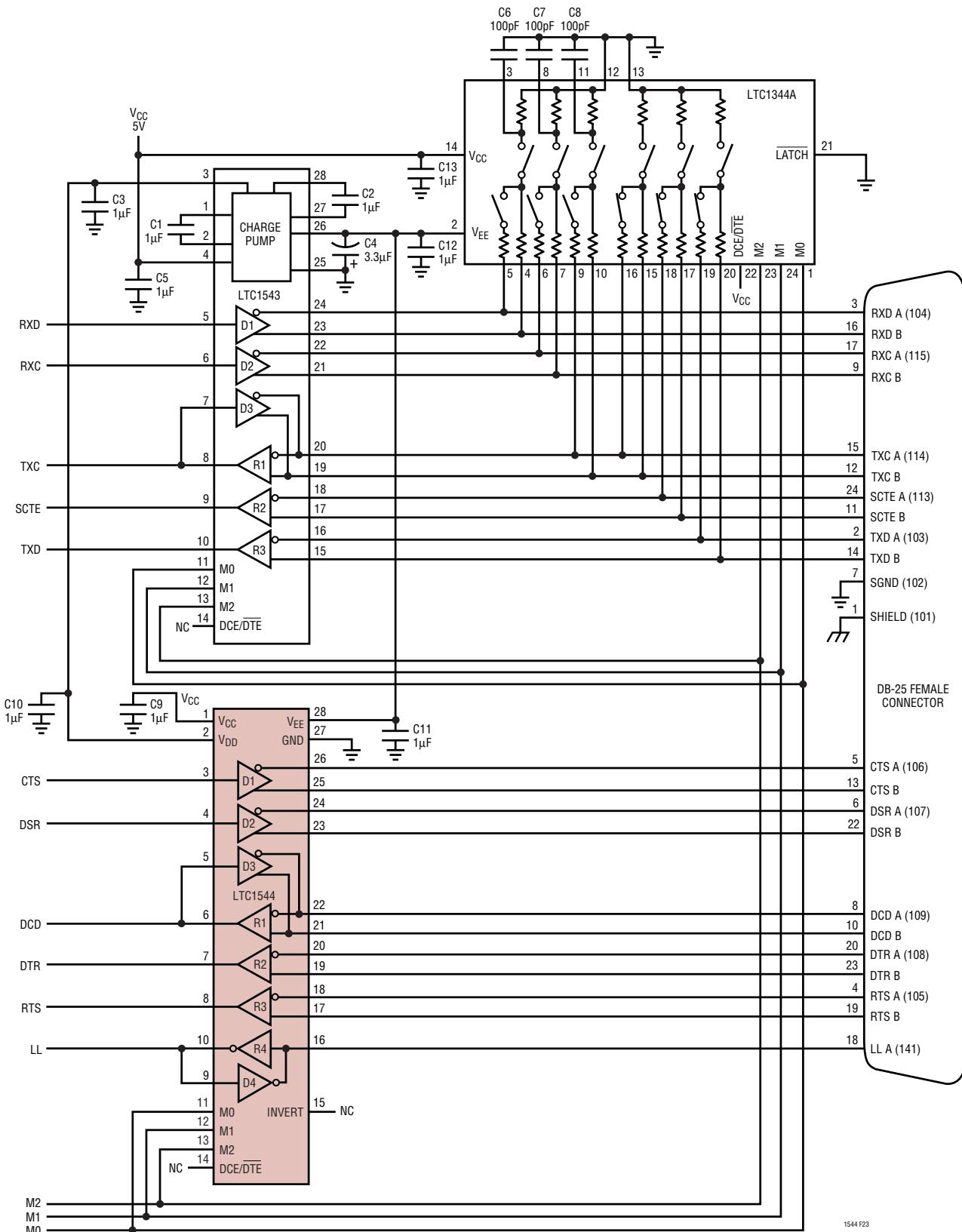
Figure 23. Controller-Selectable DCE Port with DB-25 Connector
