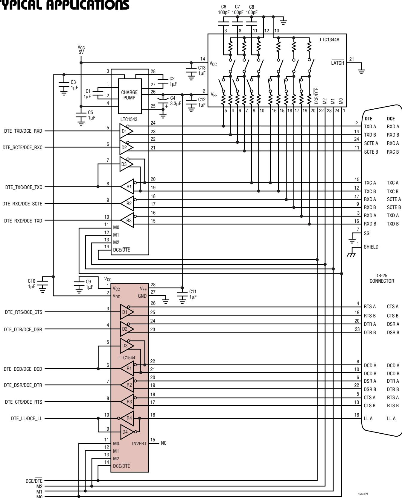
Figure 24. Controller-Selectable Multiprotocol DTE/DCE Port with DB-25 Connector
