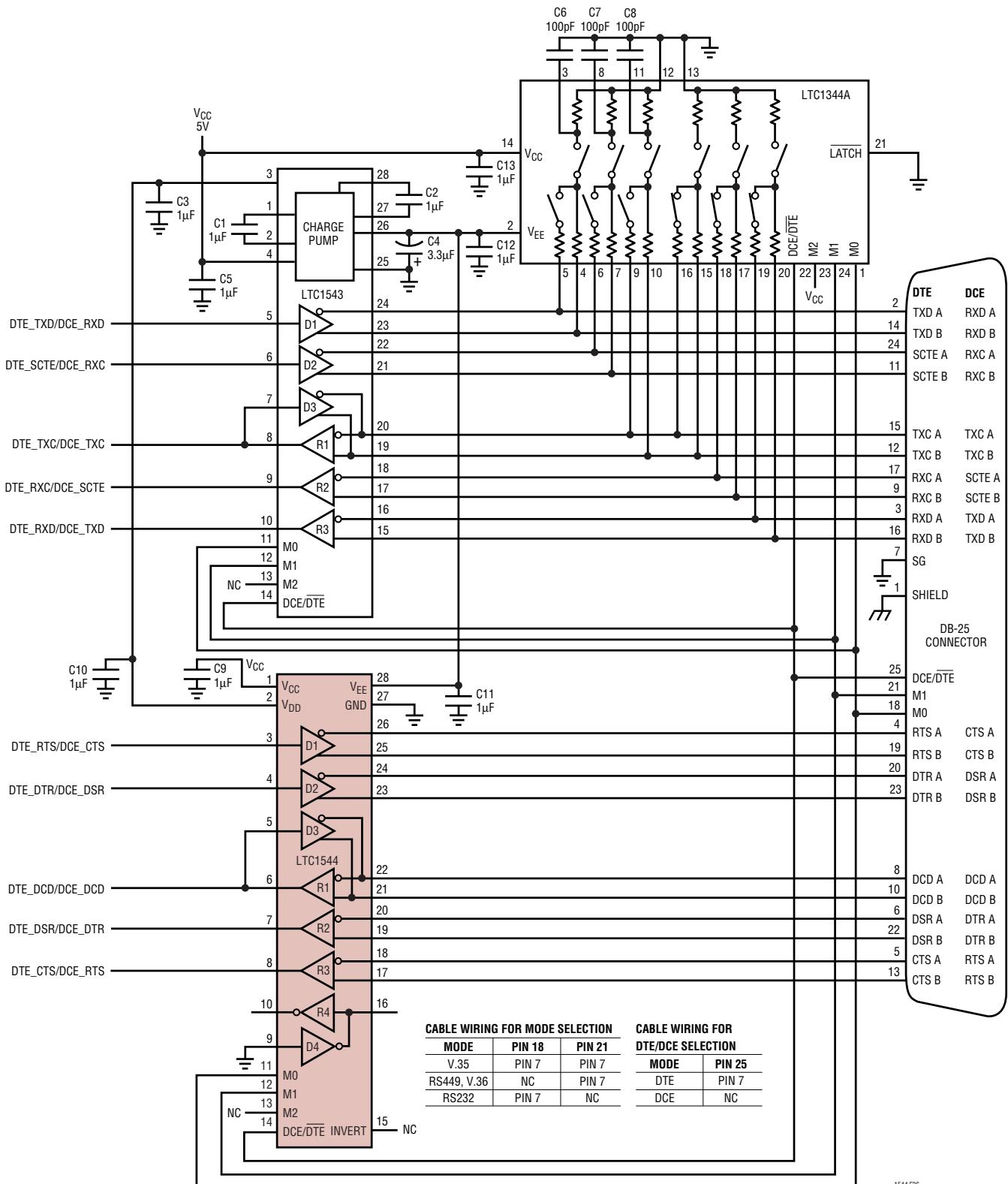
Figure 26. Cable-Selectable Multiprotocol DTE/DCE Port with DB-25 Connector
