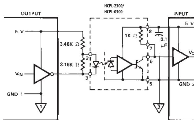
**Figure 14.** Series drive from open collector TTL/LSTTL units.
