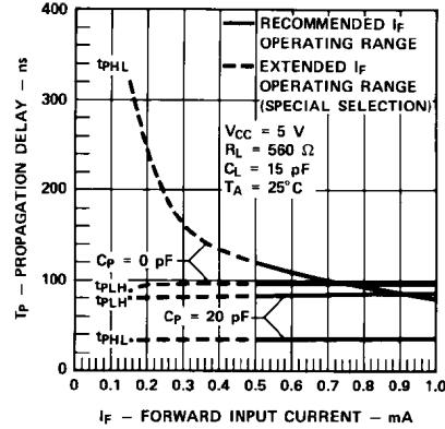
Figure 6. Typical propagation delay vs. forward current.
