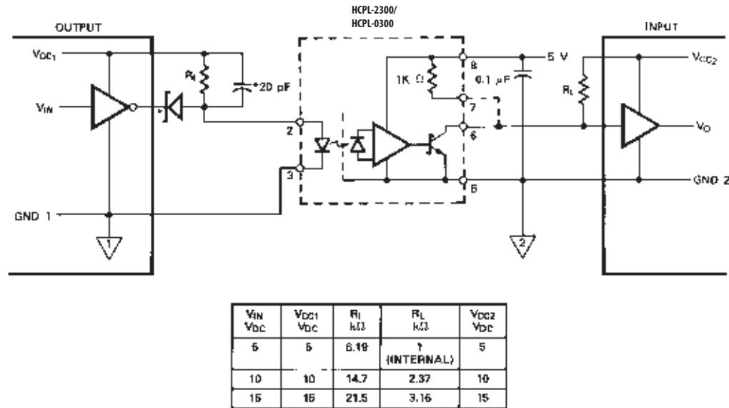
\*SCHOTTKY DIODE (HP 5062-2800, OR EQUIVALENT) AND 20 pF CAPACITOR ARE NOT REQUIRED FOR UNITS WITH OPEN COLLECTOR OUTPUT
