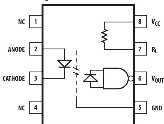
A 0.1 pF bypass capacitor must be connected between pins 5 and 8.
