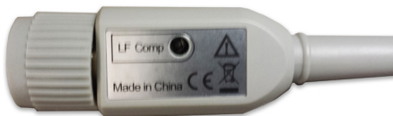
Figure 2. Low-frequency compensation adjustment (for N2840A/41A/42A/43A/53A)
