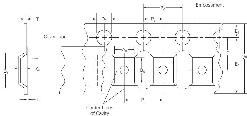
Figure A30 — EIA Referenced Reel Dimensions for AHS/ASMD/femtoASMDC/picoASMDC/nanoASMDC/microASMD/miniASMDC/ASMDC/nanoASMDCH PolySwitch Automotive Devices
