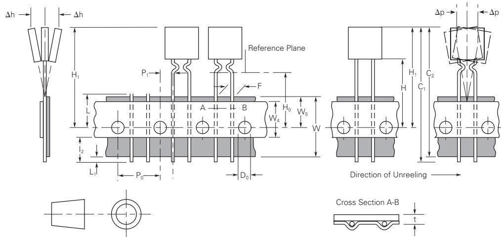
Figure A28 — EIA Referenced Reel Dimensions for AGRF/AHRF/AHEF PolySwitch Automotive Devices
