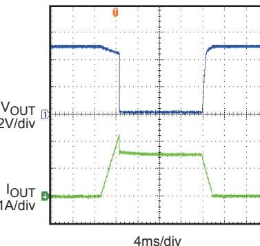
**TYPICAL PERFORMANCE CHARACTERISTICS(continued)** $V_{IN}=5V$ ,  $C_L=1\mu F$ ,  $T_a=25^\circ C$ , for only one channel, unless otherwise noted.Ramped Load
