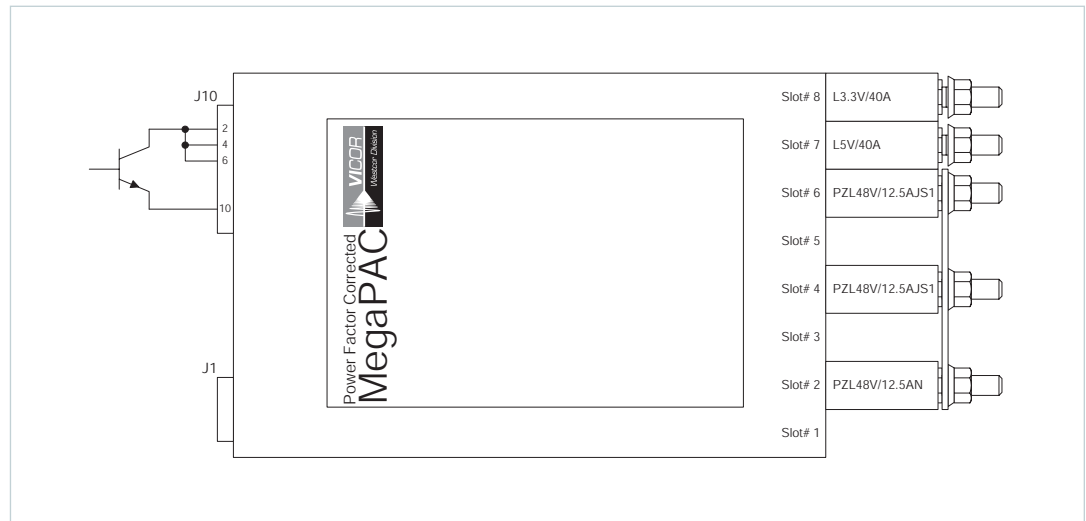
Figure 6 Enable / disable control of Maxi Arrays
