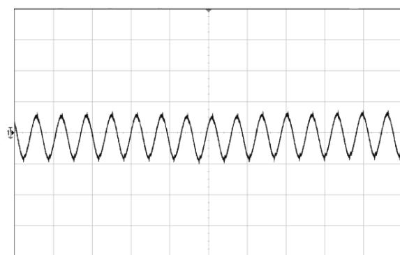
Figure 3 Input reflected ripple current (5μs/div, 10mA/div), see Figure 14 for test configuration
