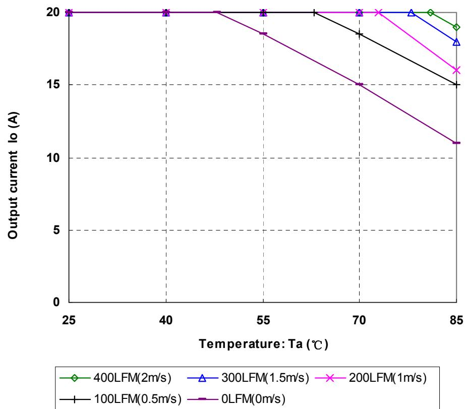
Figure 17 Output power derating, 24V<sub>in</sub>, air flowing across the converter from pin 3 to pin 1
