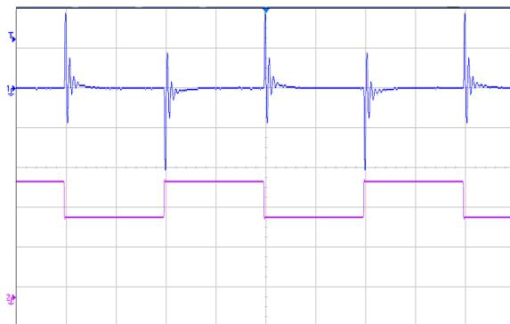
Figure 5 Dynamic response for 25% load step (50% ~ 75% ~ 50%) and 1A/ $\mu$ s slew rate, (2ms/div), see Figure 10 for test configuration; CH1-output voltage (50mv/div); CH2- output current (5A/div)
