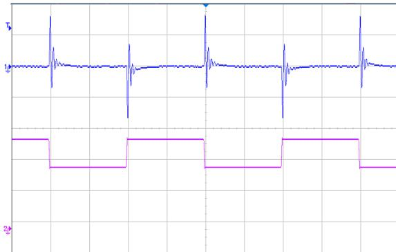
Figure 4 Dynamic response for 25% load step (50% ~ 75% ~ 50%) and 0.1A/ $\mu$ s slew rate, (2ms/div), see Figure 10 for test configuration; CH1-output voltage (50mv/div); CH2- output current (5A/div)
