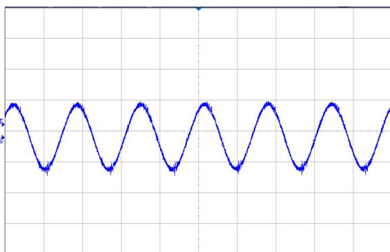
Figure 2 Output ripple & noise (2μs/div, 5mV/div), see Figure 14 for test configuration
