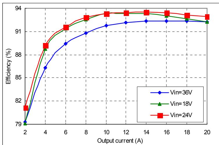
Figure 1 Efficiency vs. output current,  $T_a=25^{\circ}\text{C}$ ,  $V_o=5\text{V}$
