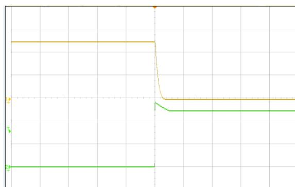
Figure 9 Output voltage shutdown by remote OFF, (500 $\mu$ s/div), see Figure 10 for test configuration; CH1-output voltage (2V/div); CH2-remote OFF voltage (2V/div)
