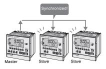
Note: Equipped on 2-circuit models.
