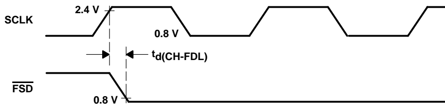
Figure 4 – 6. Slave SCLK to \overline{\text{FSD}} Timing
