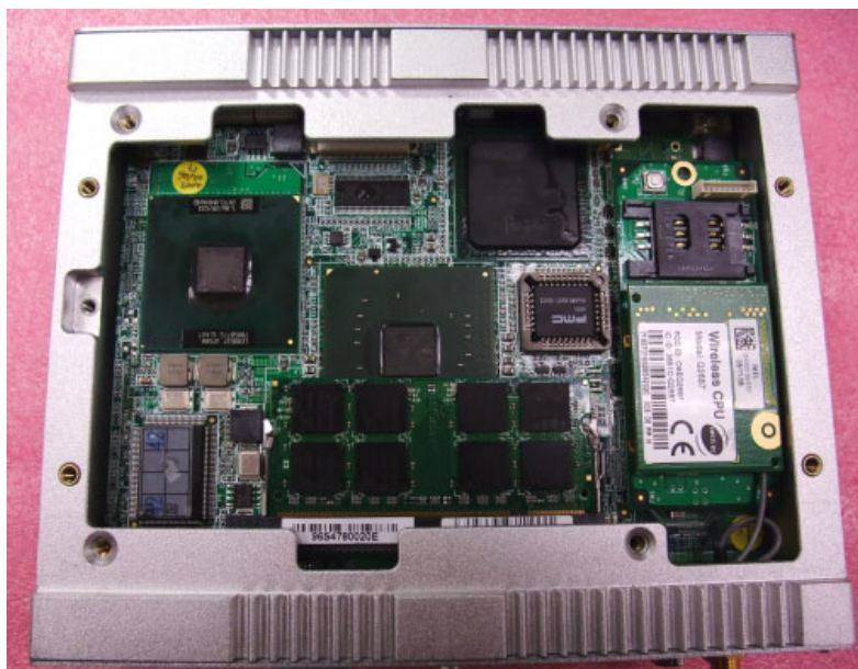
Figure 5.7 Installation AMO-EDGE on ARK-1388V
