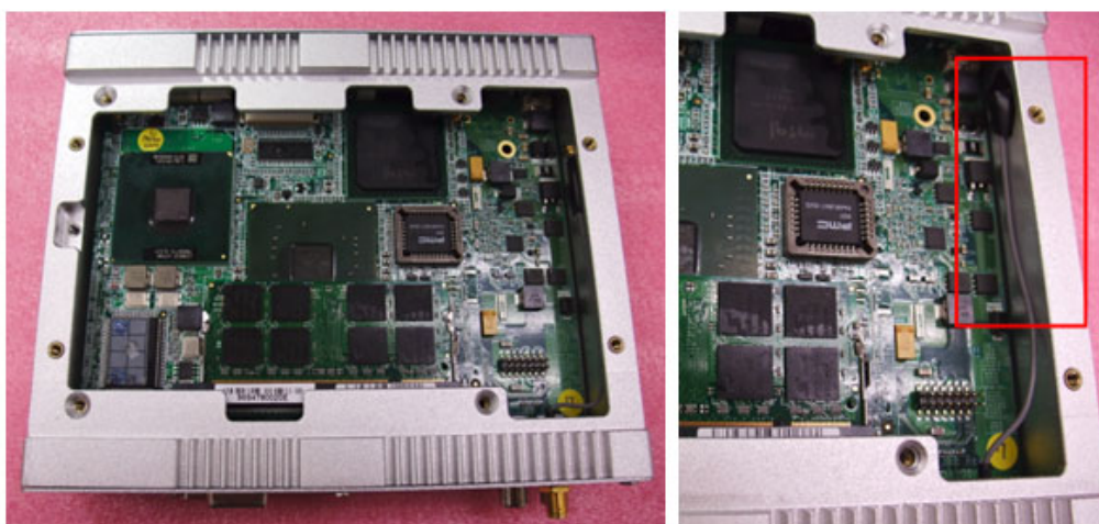
Figure 5.4 GPRS/EDGE SMA cable internally
