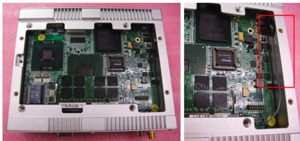
Figure 5.11 UMTS/HSDPA SMA cable internally
