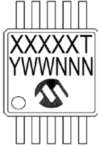
10-Lead MSOP (3x3 mm)
