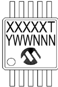
10-Lead MSOP (3x3 mm)
