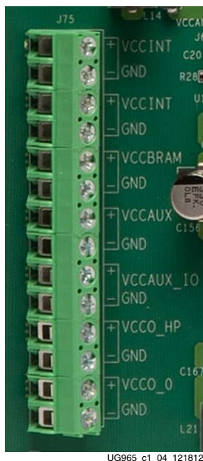
Figure 1-4: Core Power Terminal Block J75
