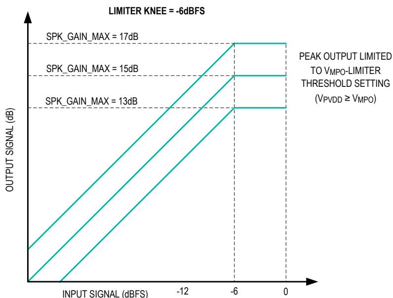
Figure 32. Example of Limiter Operation with the BDE Inactive
