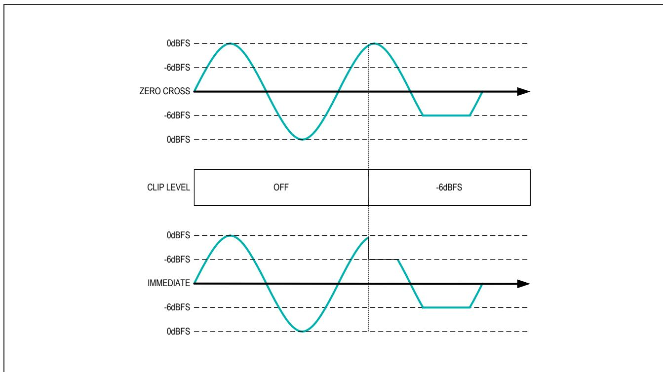
Figure 37. Clipper Example with -6dBFS Threshold
