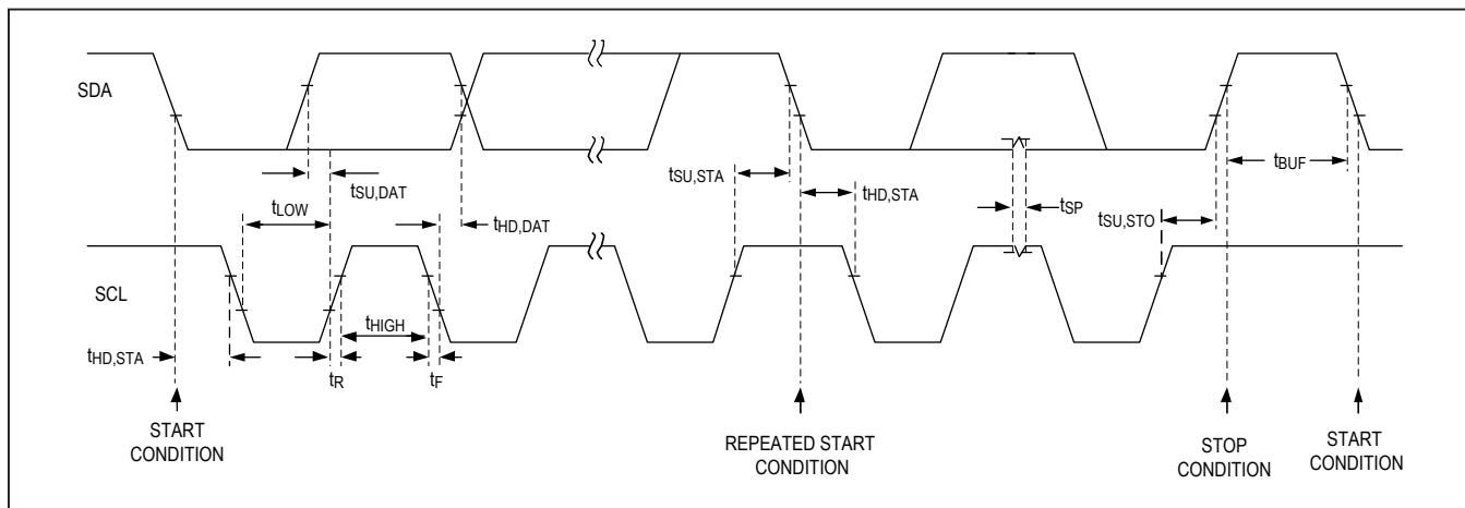
Figure 5. I<sup>2</sup>C Timing
