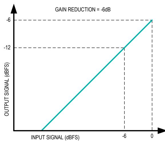
Figure 35. Gain Reduction Profile Example with -6dB Setting
