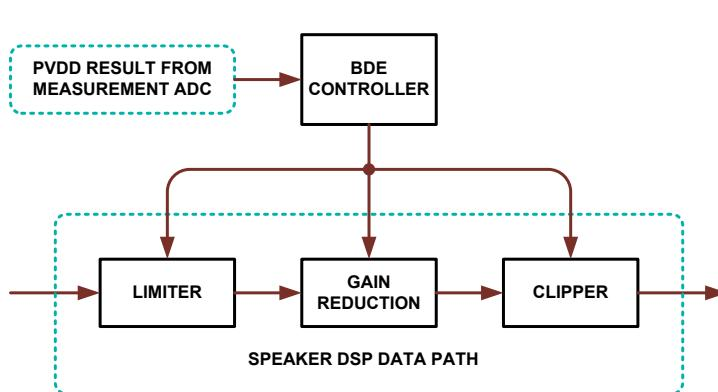
Figure 33. BDE Block Diagram
