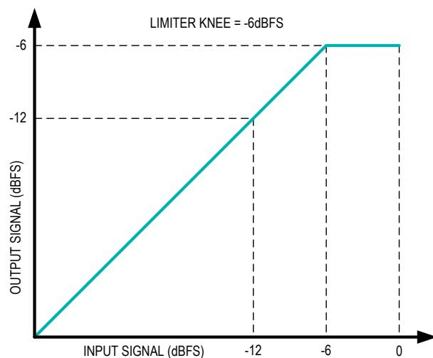
Figure 36. Limiter Profile Example with -6dBFS Knee Level
