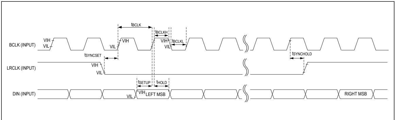
Figure 1. I<sup>2</sup>S Audio Interface Timing Diagram
