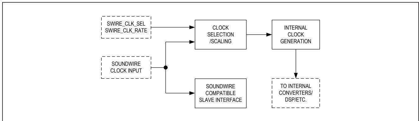
Figure 21. Internal Clock Generation in SoundWire Control Mode
