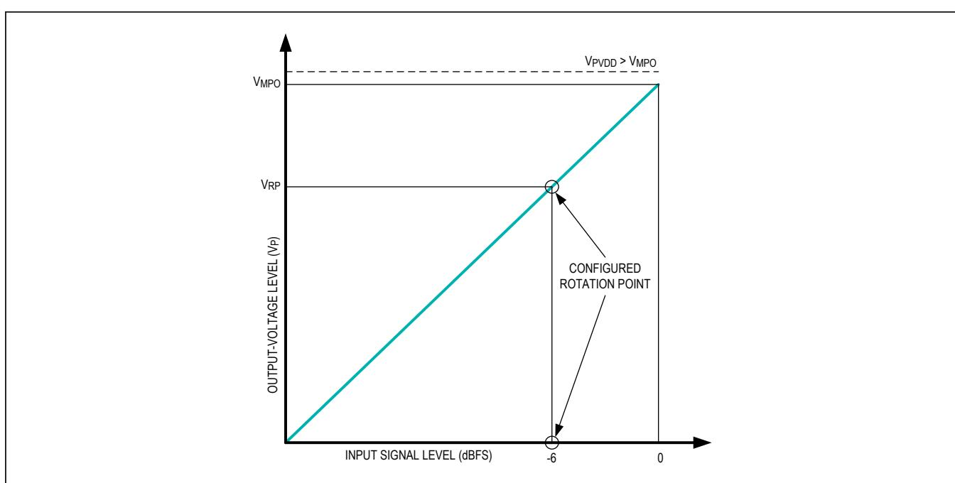
Figure 25. Example of DHT in Mode 1 Operation
