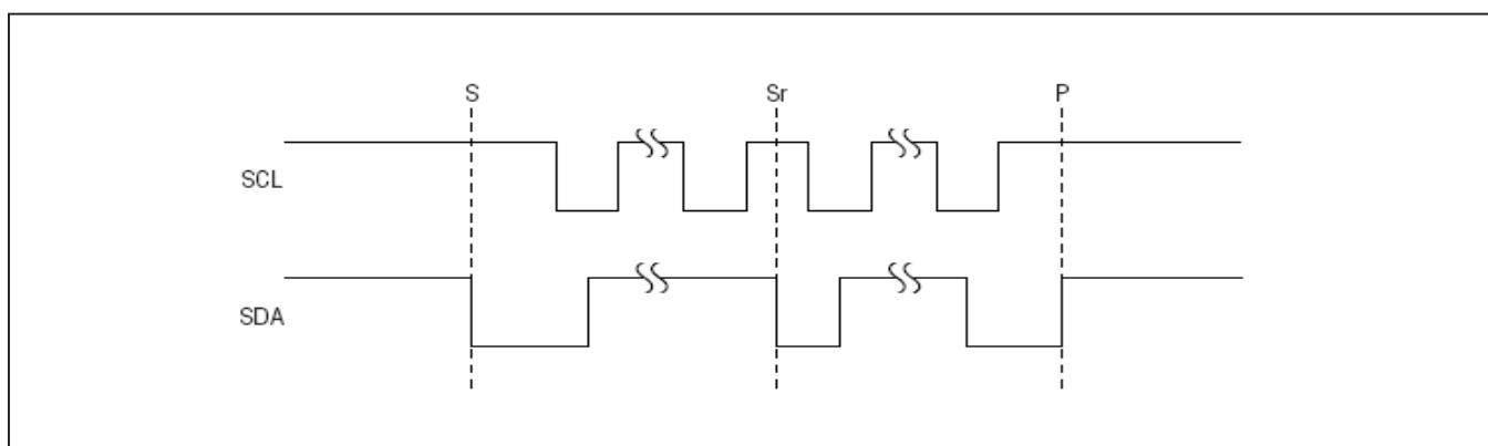
*Figure 10. START, STOP, and REPEATED START Conditions*
