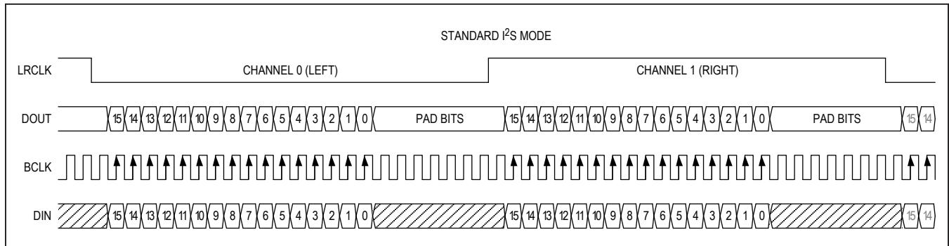
Figure 16. Standard I<sup>2</sup>S Mode Data Format Example (16-Bit Data Word, 24-Bit Channel Length)
