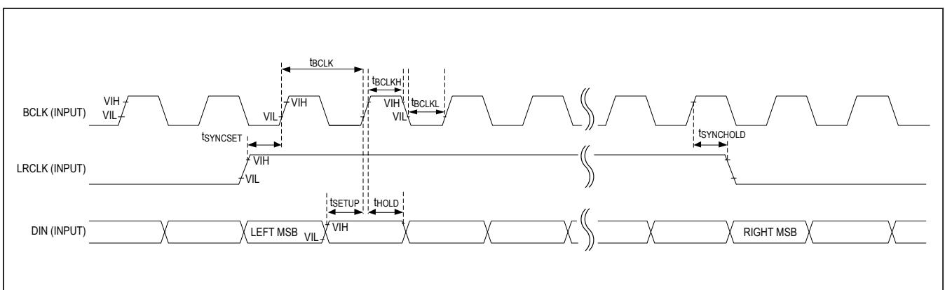
Figure 2. Left-Justified Audio Interface Timing Diagram
