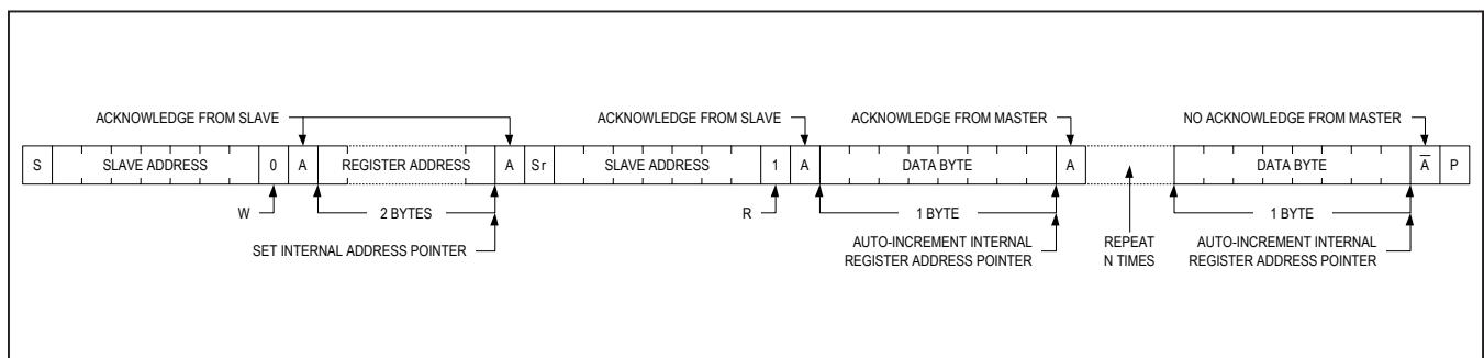
Figure 15. Reading n-Bytes of Data from the Slave
